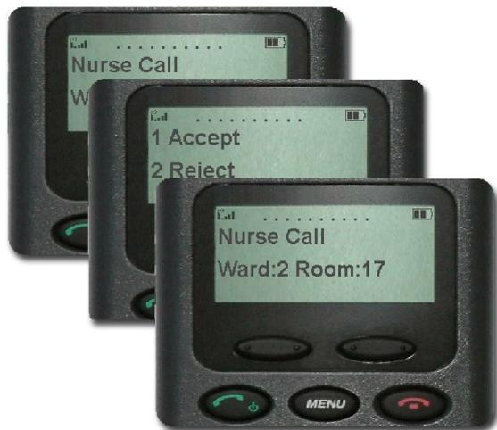
We typically connect to modern nurse call systems via the serial ports which are either RS232 or RS485, when a call is raised the nurse call outputs the relevant message via the serial port. The BlueSky Application Gateway is continuously monitoring the nurse call system serial port for all events.
